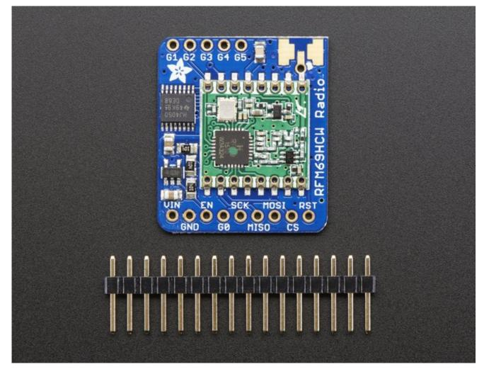
All radios are sold individually and can only talk to radios of the same part number. E.g. RFM69 900 MHz can only talk to RFM69 900 MHz, LoRa 433 MHz can only talk to LoRa 433, etc.
