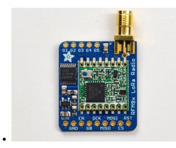
The SMA connector 'slides on' the top of the PCB
