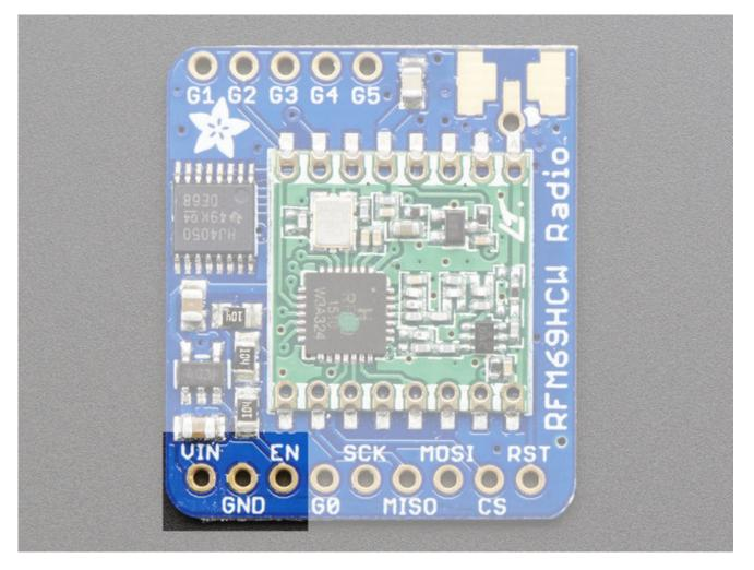
The left-most pins are used for power
