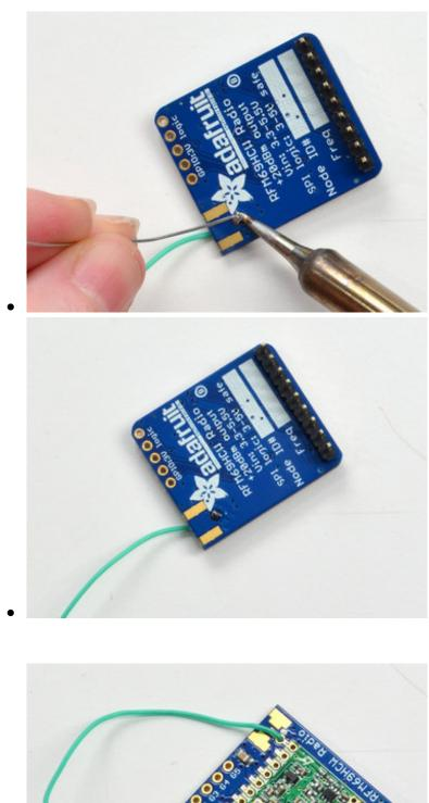
Strip a mm or two off the end of the wire, tin and solder into the **ANT** pad.
