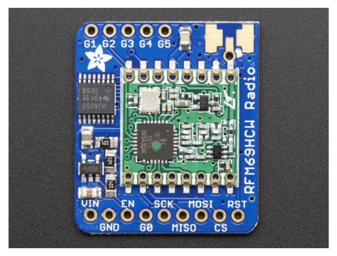
Both RFM69 and RFM9x LoRa breakouts have the exact same pinouts. The silkscreen will say RFM69HCW or LoRa depending on which variant you have. If there's a green or blue dot on top of the module, its 900 MHz. If there's a red dot, its 433 MHz
