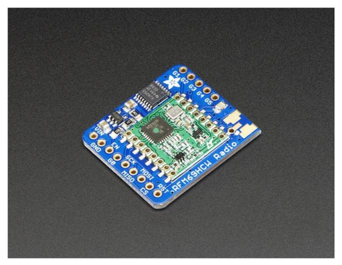
Also, these packet radios are simpler than WiFi or BLE, you dont have to associate, pair, scan, or worry about connections. All you do is send data whenever you like, and any other modules tuned to that same frequency (and, with the same encryption key) will receive. The receiver can then send a reply back. The modules do packetization, error correction and can also auto-retransmit so its not like you have worry about *everything* but less power is wasted on maintaining a link or pairing.
