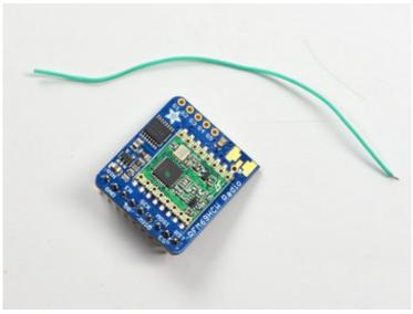
Cut a stranded or solid core wire the the proper length for the module/frequency
