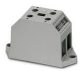
Device terminal block, Connection method: Screw connection, Number of positions: 2, Cross section: 0.75 mm² - 35 mm², AWG: 18 - 2, Width: 34.8 mm, Height: 44.9 mm, Color: gray, Mounting type: Screw mounting
