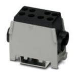
Trunk line branch terminal, Connection method: Screw connection, Screw connection, Number of connections: 4, Number of positions: 1, Cross section: 10 mm² - 35 mm², AWG: 8 - 2, Width: 27 mm, Color: black, Mounting type: NS 35/7,5, NS 35/15
