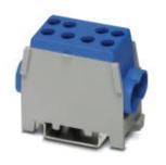
Trunk line branch terminal, Connection method: Screw connection, Screw connection, Number of connections: 4, Number of positions: 1, Cross section: 10 mm<sup>2</sup> - 35 mm<sup>2</sup>, AWG: 8 - 2, Width: 27 mm, Color: blue, Mounting type: NS 35/7,5, NS 35/15
