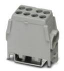
Trunk line branch terminal, Connection method: Screw connection, Screw connection, Number of connections: 4, Number of positions: 1, Cross section: 1.5 mm² - 25 mm², AWG: 8 - 2, Width: 23 mm, Color: gray, Mounting type: NS 35/7,5, NS 35/15
