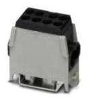
Trunk line branch terminal, Connection method: Screw connection, Screw connection, Number of connections: 4, Number of positions: 1, Cross section: 1.5 mm<sup>2</sup> - 25 mm<sup>2</sup>, AWG: 8 - 2, Width: 23 mm, Color: black, Mounting type: NS 35/7,5, NS 35/15
