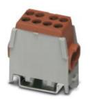
Trunk line branch terminal, Connection method: Screw connection, Screw connection, Number of connections: 4, Number of positions: 1, Cross section: 1.5 mm<sup>2</sup> - 25 mm<sup>2</sup>, AWG: 8 - 2, Width: 23 mm, Color: brown, Mounting type: NS 35/7,5, NS 35/15
