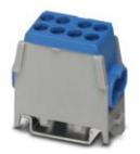
Trunk line branch terminal, Connection method: Screw connection, Screw connection, Number of connections: 4, Number of positions: 1, Cross section: 1.5 mm² - 25 mm², AWG: 8 - 2, Width: 23 mm, Color: blue, Mounting type: NS 35/7,5, NS 35/15
