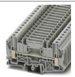
Feed-through terminal block, Connection method: Screw connection, Cross section: 0.2 mm<sup>2</sup> -10 mm<sup>2</sup>, AWG: 24 - 8, Width: 8.2 mm, Mounting type: NS 35/7,5, NS 35/15, NS 32, Color: gray
