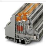
Knife disconnect terminal block, With test socket screws for insertion of test plugs, nom. voltage: 400 V, nominal current: 10 A, connection method: Screw connection, cross section: 0.2 mm<sup>2</sup> - 4 mm<sup>2</sup>, AWG: 24 - 12, length: 93 mm, width: 6.2 mm, color: gray, mounting: NS 35/7,5, NS 35/15, NS 32, nom. voltage: 400 V
