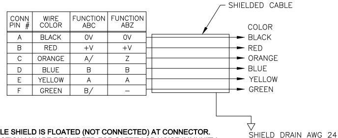
WARNING: CABLE SHIELD IS FLOATED (NOT CONNECTED) AT CONNECTOR. SHIELD CONNECTION MAY BE REQUIREED FOR SAFETY OR NOISE IMMUNITY.
