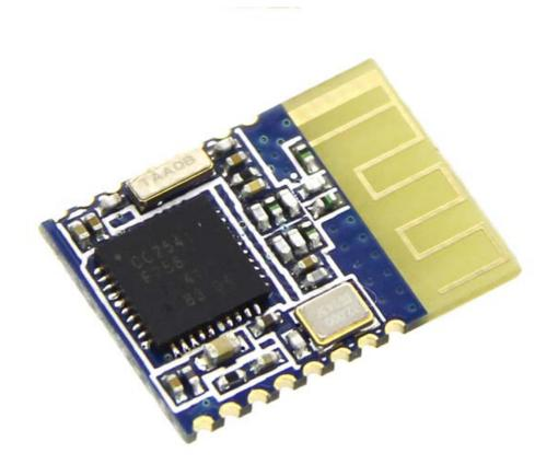
This is a SMD BLE module used in our BLE Bee and Xadow BLE. It is based on TI CC2541 chip, enables robust network nodes to be built with low total bill-of-material costs and highly suited for ultralow power consumption systems. The module is small and easy to use, with the preprogrammed firmware of manufacturer, you could quickly build BLE communications via its AT command. Supporting BLE communications with iphone, ipad and Android 4.3.
