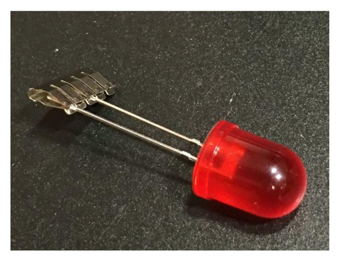
Each clip can handle at least a hundred plugs and unplugs before the springiness of the clip slowly weakens and eventually stops gripping so well. You'll know when the breadboard needs replacing because you wont feel the clip gripping onto the part when you press it in.
