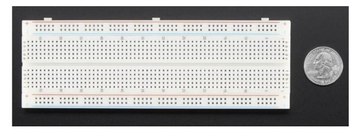
These "Solder-less" Breadboards are incredibly handy for building circuits. They are durable and reusable and have tons of work space. They not only hold your parts steady, a breadboard also has *internal wiring* to make connections super fast.
