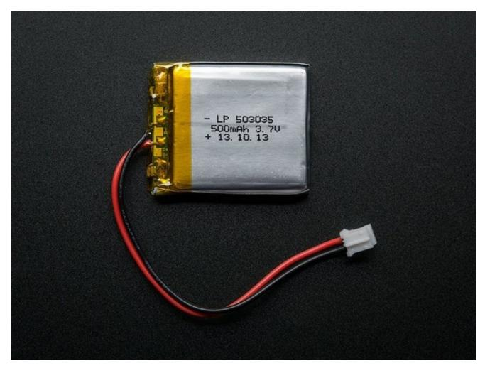
Lithium ion polymer (also known as 'lipo' or 'lipoly') batteries are thin, light and powerful. The output ranges from 4.2V when completely charged to 3.7V. This battery has a capacity of 500mAh for a total of about 1.9 Wh.
