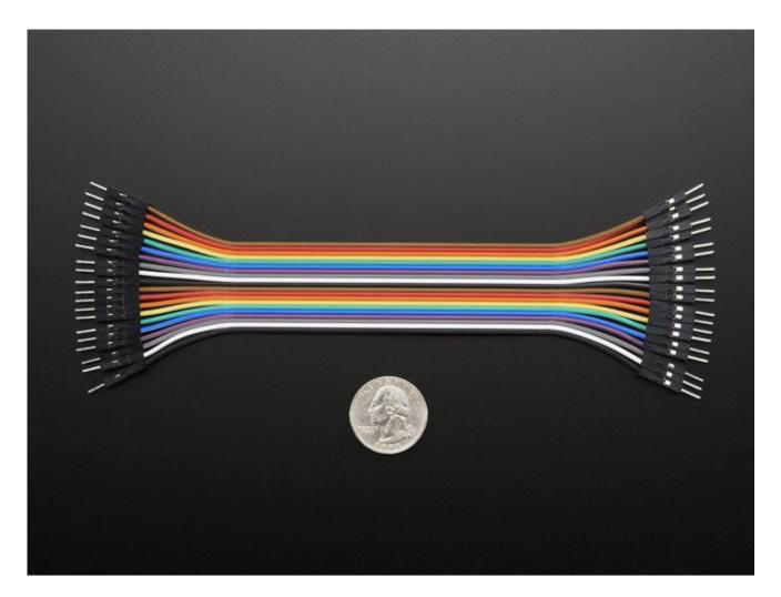
Each version comes in a 'strip' of 20 (2 pieces of each of ten rainbow colors). They have 0.1" male header contacts on either end and fit cleanly next to each other on standard-pitch 0.1" (2.54mm) breadboards. The best part is they come in a 20-pin ribbon cable. You can always pull the ribbon wires off to make individual jumpers, or keep them together to make neatly organized wire harnesses.
