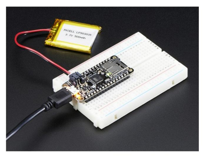
If the battery is plugged into the Feather and the USB cable is connected to a computer or power supply it will automatically recharge the battery. The yellow LED will light up to let you know. When the yellow light turns off, the battery is done charging
