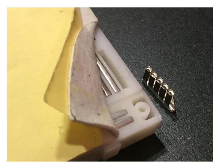
These little teeth are great at gripping onto electronic parts. When a part is pushed into the breadboard, the clip pushes open and grabs onto the metal leg. Any other parts that are plugged into the other 4 teeth are thus electrically connected together
