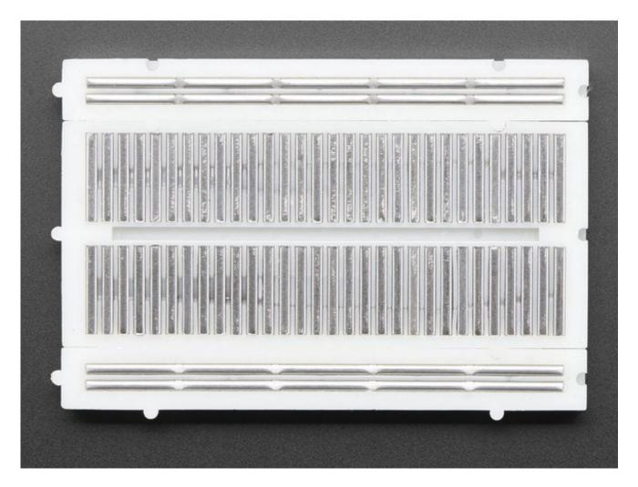
If you pulled the metal parts out with pliers (again, don't do this yourself!) You'd see each one is a metal clip with little teeth. The rows have 5 teeth - one for each hole on the top of the breadboard. (The power rails have 50 teeth)
