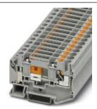
Test disconnect terminal block, With test socket screws for insertion of test plugs, connection method: Pushin connection, Screw connection, cross section: 0.5 mm² - 10 mm², AWG: 20 - 10, width: 8.2 mm, color: gray, mounting: NS 35/7,5, NS 35/15
