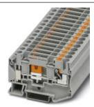
Test disconnect terminal block, connection method: Push-in connection, Screw connection, cross section: 0.5 mm² - 10 mm², AWG: 20 - 10, width: 8.2 mm, color: gray, mounting: NS 35/7,5, NS 35/15
