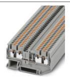
Feed-through terminal block, Connection method: Push-in connection, Number of connections: 4, Cross section: 0.14 mm² - 4 mm², AWG: 26 - 12, Width: 5.2 mm, Height: 35.3 mm, Color: white, Mounting type: NS 35/7,5, NS 35/15
