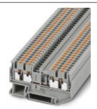
Feed-through terminal block, Connection method: Push-in connection, Number of connections: 4, Cross section: 0.14 mm² - 4 mm², AWG: 26 - 12, Width: 5.2 mm, Height: 35.3 mm, Color: green, Mounting type: NS 35/7,5, NS 35/15
