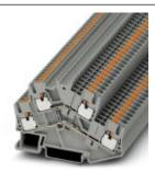
Double-level terminal block, Cross section: 0.14 mm<sup>2</sup> - 4 mm<sup>2</sup>, AWG: 26 - 12, Connection type: Push-in connection, Width: 5.2 mm, Color: gray, Mounting type: NS 35/7,5, NS 35/15
