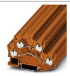
Double-level terminal block, Cross section: 0.14 mm<sup>2</sup> - 4 mm<sup>2</sup>, AWG: 26 - 12, Connection type: Push-in connection, Width: 5.2 mm, Color: orange, Mounting type: NS 35/7,5, NS 35/15
