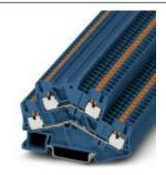
Double-level terminal block, Cross section: 0.14 mm<sup>2</sup> - 4 mm<sup>2</sup>, AWG: 26 - 12, Connection type: Push-in connection, Width: 5.2 mm, Color: blue, Mounting type: NS 35/7,5, NS 35/15
