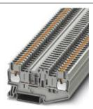
Disconnect terminal block, Connection type: Push-in connection, Cross section: 0.14 mm² - 4 mm², AWG: 26 - 12, Nominal current: 16 A, Nominal voltage: 400 V, Length: 70.1 mm, Width: 5.2 mm, Color: gray, Assembly: NS 35/7,5, NS 35/15
