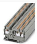
Component terminal block, with integrated 1N4007 diode, nom. voltage: 800 V, nominal current: 0.5 A, connection method: Push-in connection, number of connections: 3, cross section:0.14 mm² - 4 mm², AWG: 26 - 12, width: 5.2 mm, color: gray, mounting type: NS 35/7,5, NS 35/15
