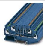
Feed-through terminal block, Cross section: 0.14 mm<sup>2</sup> - 4 mm<sup>2</sup>, AWG: 26 - 12, Connection type: Push-in connection, Width: 5.2 mm, Color: blue, Mounting type: NS 35/7,5, NS 35/15
