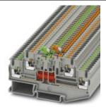
Disconnect terminal block, Connection type: Push-in connection, Cross section: 0.14 mm² - 4 mm², AWG: 26 - 12, Nominal current: 16 A, Nominal voltage: 400 V, Length: 92.4 mm, Width: 5.2 mm, Color: blue, Assembly: NS 35/7,5, NS 35/15
