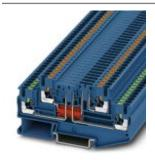
Disconnect terminal block, with isolating plug, Connection type: Push-in connection, Cross section: 0.14 mm<sup>2</sup> - 4 mm<sup>2</sup>, AWG: 26 - 12, Nominal current: 16 A, Nominal voltage: 400 V, Length: 92.4 mm, Width: 5.2 mm, Color: blue, Assembly: NS 35/7,5, NS 35/15
