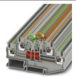
Disconnect terminal block, Connection type: Push-in connection, Cross section: 0.14 mm² - 4 mm², AWG: 26 - 12, Nominal current: 16 A, Nominal voltage: 400 V, Length: 92.4 mm, Width: 5.2 mm, Color: gray, Assembly: NS 35/7,5, NS 35/15
