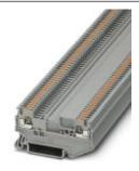
Knife disconnect terminal block, same shape as disconnect terminal block, Connection type: Push-in connection, Cross section: 0.14 mm<sup>2</sup> - 1.5 mm<sup>2</sup>, AWG: 26 - 14, Nominal current: 17.5 A, Nominal voltage: 400 V, Length: 58.9 mm, Width: 3.5 mm, Color: gray, Assembly: NS 35/7,5, NS 35/15
