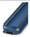
Knife disconnect terminal block, same shape as disconnect terminal block, Connection type: Push-in connection, Cross section: 0.14 mm<sup>2</sup> - 1.5 mm<sup>2</sup>, AWG: 26 - 14, Nominal current: 17.5 A, Nominal voltage: 400 V, Length: 58.9 mm, Width: 3.5 mm, Color: blue, Assembly: NS 35/7,5, NS 35/15
