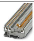
Knife disconnect terminal block, Connection type: Push-in connection, Cross section: 0.14 mm² - 1.5 mm², AWG: 26 - 14, Nominal current: 10 A, Nominal voltage: 400 V, Length: 67.8 mm, Width: 3.5 mm, Color: gray, Assembly: NS 35/7,5, NS 35/15
