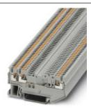
Disconnect terminal block, Connection type: Push-in connection, Cross section: 0.14 mm² - 1.5 mm², AWG: 26 - 14, Nominal current: 10 A, Nominal voltage: 400 V, Length: 67.8 mm, Width: 3.5 mm, Color: gray, Assembly: NS 35/7,5, NS 35/15
