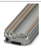
Feed-through terminal block, same shape as disconnect terminal block, Connection method: Push-in connection, Cross section: 0.14 mm² - 1.5 mm², AWG: 26 - 14, Width: 3.5 mm, Height: 30.5 mm, Color: gray, Mounting type: NS 35/7,5, NS 35/15
