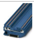
Feed-through terminal block, same shape as disconnect terminal block, Connection method: Push-in connection, Cross section: 0.14 mm² - 1.5 mm², AWG: 26 - 14, Width: 3.5 mm, Height: 30.5 mm, Color: blue, Mounting type: NS 35/7,5, NS 35/15
