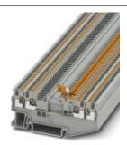
Knife disconnect terminal block, Connection type: Push-in connection, Cross section: 0.14 mm² - 1.5 mm², AWG: 26 - 14, Nominal current: 10 A, Nominal voltage: 400 V, Length: 76.9 mm, Width: 3.5 mm, Color: gray, Assembly: NS 35/7,5, NS 35/15
