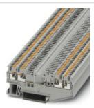
Disconnect terminal block, Connection type: Push-in connection, Cross section: 0.14 mm² - 1.5 mm², AWG: 26 - 16, Nominal current: 10 A, Nominal voltage: 400 V, Length: 76.9 mm, Width: 3.5 mm, Color: gray, Assembly: NS 35/7,5, NS 35/15
