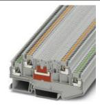
Feed-through terminal block, Connection method: Push-in connection, Cross section: 0.14 mm² - 1.5 mm², AWG: 26 - 14, Width: 3.5 mm, Height: 41.1 mm, Color: gray, Mounting type: NS 35/7,5, NS 35/15
