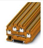
Double-level terminal block, connection method: Push-in connection, cross section: 0.14 mm<sup>2</sup> - 4 mm<sup>2</sup>, AWG: 26 - 12, width: 5.2 mm, color: orange, mounting type: NS 35/7,5, NS 35/15
