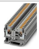
Feed-through terminal block, Connection method: Push-in connection, Cross section: 0.5 mm<sup>2</sup> - 10 mm<sup>2</sup>, AWG: 20 - 8, Width: 8.2 mm, Height: 42.2 mm, Color: gray, Mounting type: NS 35/7,5, NS 35/15
