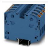
High-current terminal block, nom. voltage: 1000 V, nominal current: 125 A, connection method: Power-Turn connection, number of connections: 2, cross section:2.5 mm² - 35 mm², AWG: 12 - 2, width: 16 mm, color: blue, mounting type: NS 35/15
