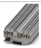
Feed-through terminal block, Connection method: Spring-cage connection, Cross section: 0.08 mm<sup>2</sup> - 1.5 mm<sup>2</sup>, AWG: 28 - 16, Width: 3.5 mm, Color: gray, Mounting type: NS 35/7,5, NS 35/15
