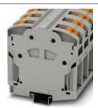
High-current terminal block, Connection method: Power-Turn connection, Number of positions: 1, Cross section: 50 mm² - 150 mm², AWG: 1/0 - 300 kcmil, Width: 31 mm, Color: gray, Mounting type: NS 35/15
