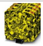
High-current terminal block, Connection method: Power-Turn connection, Number of positions: 1, Cross section: 50 mm<sup>2</sup> - 150 mm<sup>2</sup>, AWG: 1/0 - 300 kcmil, Width: 31 mm, Color: black/yellow, Mounting type: NS 35/15
