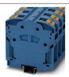
High-current terminal block, Connection method: Power-Turn connection, Number of positions: 1, Cross section: 50 mm² - 150 mm², AWG: 1/0 - 300 kcmil, Width: 31 mm, Color: blue, Mounting type: NS 35/15
