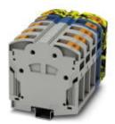
High-current terminal block, Blocked, Connection method: Power-Turn connection, Number of positions: 4, Cross section: 50 mm² - 150 mm², AWG: 1/0 - 300 kcmil, Width: 124 mm, Color: gray/black-yellow, Mounting type: NS 35/15
