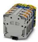
High-current terminal block, Blocked, Connection method: Power-Turn connection, Number of positions: 5, Cross section: 50 mm² - 150 mm², AWG: 1/0 - 300 kcmil, Width: 155 mm, Color: gray/blue/black-yellow, Mounting type: NS 35/15
