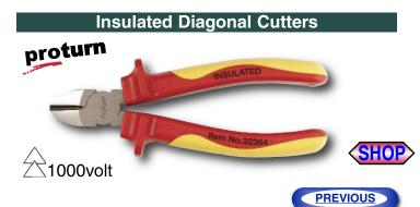
323 Proturn Insulated Diagonal Cutters. Insulation According to VDE 0682/part 201, DIN 7437, EN/IEC 60900, ASTM F-1505-01, NFPA70E, 1000 volt rated. Individually Tested. DIN ISO 5745 Pliers drop-forged from special tool steel, individually high frequency induction hardened, chrome and nickel plated, mirror polished. Proturn ergo soft grip handles for maximum comfort.
