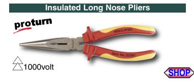
323Proturn Insulated Long Nose Pliers. Insulation According<br/>to VDE 0682/part 201, DIN 7437, EN/IEC 60900, ASTM F-1505-01,<br/>NFPA70E, 1000 volt rated. Individually Tested. DIN ISO 5745Pliers drop-forged from special tool steel, individually high frequency<br/>induction hardened, chrome and nickel plated, mirror polished. Proturn<br/>ergo soft grip handles for maximum comfort.
