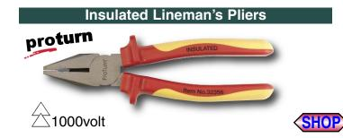
323Proturn Insulated Lineman's Pliers. Insulation According<br/>to VDE 0682/part 201, DIN 7437, EN/IEC 60900, ASTM F-1505-01,<br/>NFPA70E, 1000 volt rated. Individually Tested. DIN ISO 5745Pliers drop-forged from special tool steel, individually high frequency<br/>induction hardened, chrome and nickel plated, mirror polished. Proturn<br/>ergo soft grip handles for maximum comfort.
