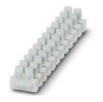
Polyamide Europe terminal strip, transparent, with wire protection, for connecting solid conductors and stranded conductors with and without ferrules with a cross section of 0.75 to 4 mm<sup>2</sup>
