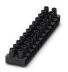
Polypropylene Europe terminal strip, black, for connecting solid conductors and stranded conductors with and without ferrules with a cross section of 0.75 to 6 mm<sup>2</sup>
