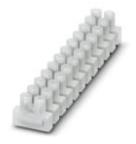
Polyamide Europe terminal strip, transparent, for connecting solid conductors and stranded conductors with ferrules with a cross section of 0.75 to 6 mm<sup>2</sup>
