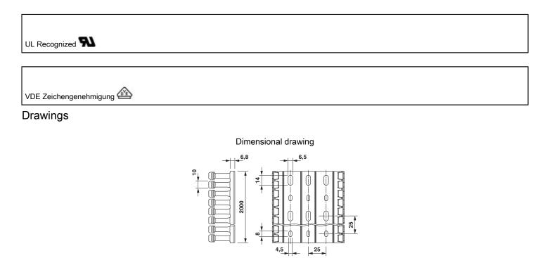
Base perforation according to DIN EN 50085
