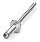
Blind rivets, Ø 2.4 mm, 8 mm sleeve length, aluminum sleeve, zinc-plated steel pin, special version with extended pin for fixing UW/RW/PW 4... (the UNIFOX-RVT M/BIT 2,4L nosepiece is required for processing)
